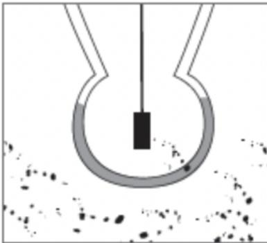
In time, particles during routine measurement can contaminate the sensor tip. Mishandled and aged solutions can also be affected.
