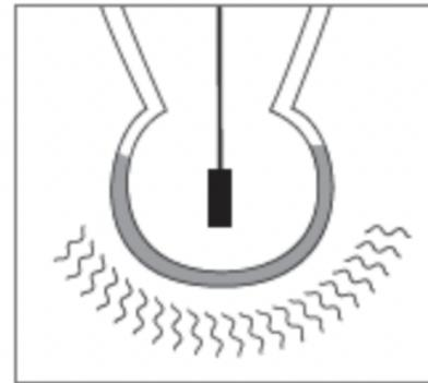
A proper cleaning and fresh solution ensures the whole surface of the sensor tip is reading correctly, ensuring an accurate calibration.
