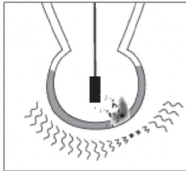
Your meter can still be calibrated even if the electrode sensor tip is not properly cleaned before calibration. If the contamination dissipates, the calibration is no longer valid and the readings are inaccurate.
